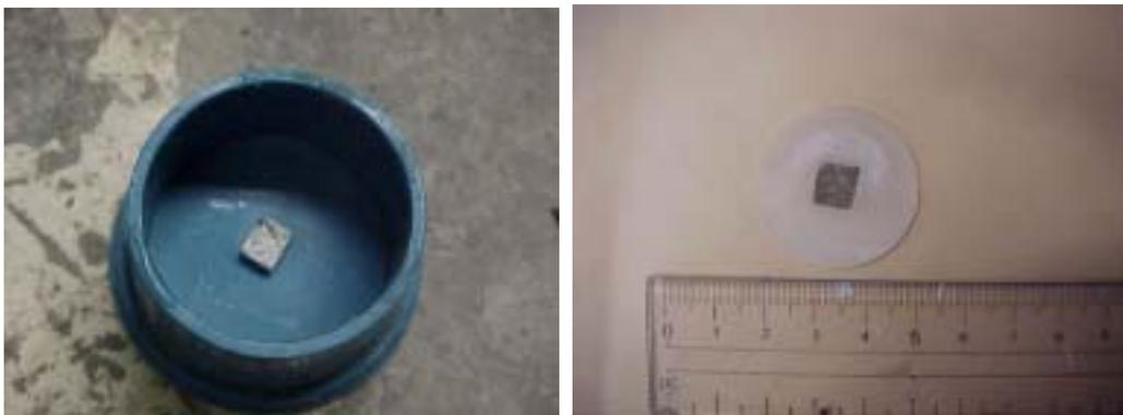
**Fig. 2.2.5** Final Test Piece Set in Hard Epoxy.
